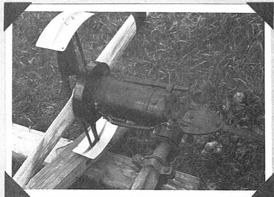
PHOTO 7. Wincharger 200 Watt - 6 Volt - Model 622 - 1950
