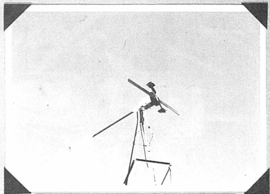
PHOTO 6. Wincharger 200 Watt - 12 Volt - Model 1222H - 1974
