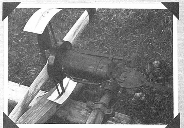
PHOTO 7. Wincharger 200 Watt - 6 Volt - Model 622 - 1950
