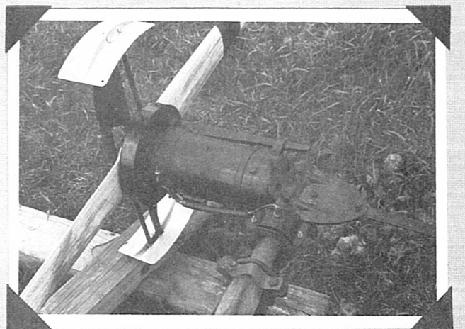
PHOTO 7. Wincharger 200 Watt - 6 Volt - Model 622 - 1950
